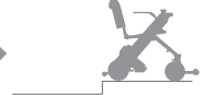
Do the same for the rear wheels to get the device over the step.
